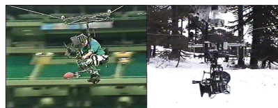
Figure 4.59 Skycam operation during the show consists of two people, with additional technical and logistical support standing by. The left operator controls camera zooming, focusing and pan/tilt. A control panel from CF Inflight installed in the production truck controls the camera's video levels. The person on the right is the pilot. He, in conjunction with the setup technical crew, enters coordinates as to ceiling, floor and flight boundary limits — in other words, the 3-D box that Skycam can fly around in. The crew also maps out no-fly zones inside the flight box, such as baskets and goal posts. During the show the pilot, via a central computer that orchestrates the operation of the four reels, flies the Skycam Spar through 3-D space. Every Skycam pilot is required to go to CF Inflight's training for certification to fly the system.
