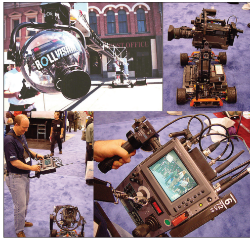
Figure 4.50 A number of companies have based a large part of their business model on getting those camera shots that make us wonder how they did that. One such company is Rollvision. Upper left is the company's basic package, which weighs 16 lbs. and allows the contained camera to roll and pan 360 degrees and tilt 180 degrees. As shown here, it can be mounted on a jib or on other interesting mounts. Bottom right shows the radio remote control of the Rollvision assembly.
