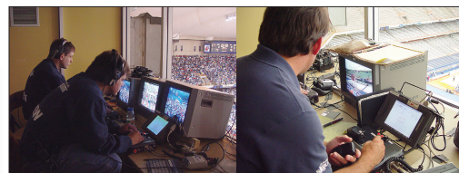
Figure 4.59 Skycam operation during the show consists of two people, with additional technical and logistical support standing by. The left operator controls camera zooming, focusing and pan/tilt. A control panel from CF Inflight installed in the production truck controls the camera's video levels. The person on the right is the pilot. He, in conjunction with the setup technical crew, enters coordinates as to ceiling, floor and flight boundary limits — in other words, the 3-D box that Skycam can fly around in. The crew also maps out no-fly zones inside the flight box, such as baskets and goal posts. During the show the pilot, via a central computer that orchestrates the operation of the four reels, flies the Skycam Spar through 3-D space. Every Skycam pilot is required to go to CF Inflight's training for certification to fly the system.
