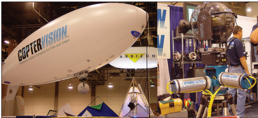
Figure 4.49 Other platforms include this 30-foot indoor blimp, which can be used outdoors if the winds are under 20mph. The Rollvision camera container is below. The system on the right is Rollvision on a camera stabilization head, which removes pitch and roll and thus automatically maintains camera horizontal. This system could be used onboard a boat, on an off-road vehicle or even on an aircraft. It mounts between the tripod and the pan/tilt head.
