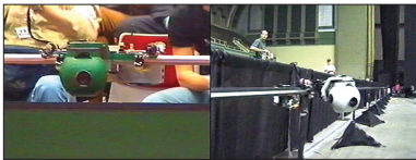
Figure 4.54 The technology and brainpower behind Steadicam didn't stop there, as Steadicam inventor Garrett Brown and crew found other specialized camera platform and aiming requirements and filled them. Here is Railcam. This device allows a camera to race up and down a tennis court, or pace the participants in track. (Source: Steadicam)
