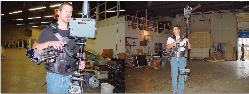
Figure 4.53 A couple examples of the latest iteration of Steadicam. This system can be configured for over the shoulder or low to the ground camera shots. The spring-loaded arm, along with the long pole with camera mass at one end and the support electronics and monitor at the other end, creates a large moment of inertia. This is how the system produces smooth camera moves. But what makes Steadicam a powerful production tool are the artists that guide it around, and often through, the action being captured. Here are two Steadicam operators honing their skills at a Steadicam workshop. Between Garrett Brown, the late Ted Churchill and a few other masters, about 2000 operators have been through "the system." Good Steadicam operators are an important part of a production, often called upon to help choreograph how a scene is shot, and the great ones are often considered on a par with the shoot's director of photography (DP).
