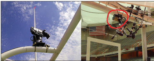
Figure 4.48 Point of view (POV) cameras. Left camera sits atop a football goal post, and the other (circled in red) is a small camera on the back of a basketball backboard. Below and behind the camera is its spidery tripod assembly, which is clamped to the backboard frame. Both cameras are remote controlled from the truck compound.
