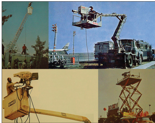
Figure 4.44 In almost every case, there must be camera locations that are above the action. For many productions, the easiest way to get a camera above the action where there isn't already a platform is to rent a lift. Although, if the need was frequent enough, an entity like Japan's NHK might own their own.
